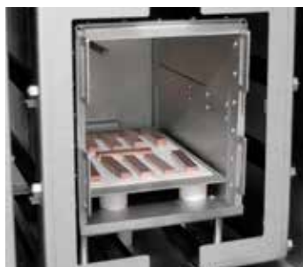
Heat treatment of copper bars under hydrogen in retort furnace VHT 8/16-MO
