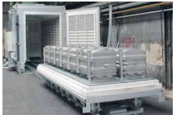
Bogie hearth furnace with gas supply system
