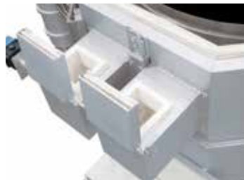
Motor-driven fresh-air and exhaust air flaps
