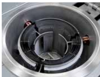
Cylindrical retort with tungsten heating
