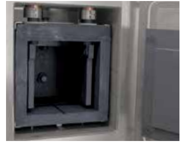
Graphite heating chamber
