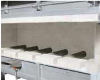
Indirect gas firing with radiation tubes
