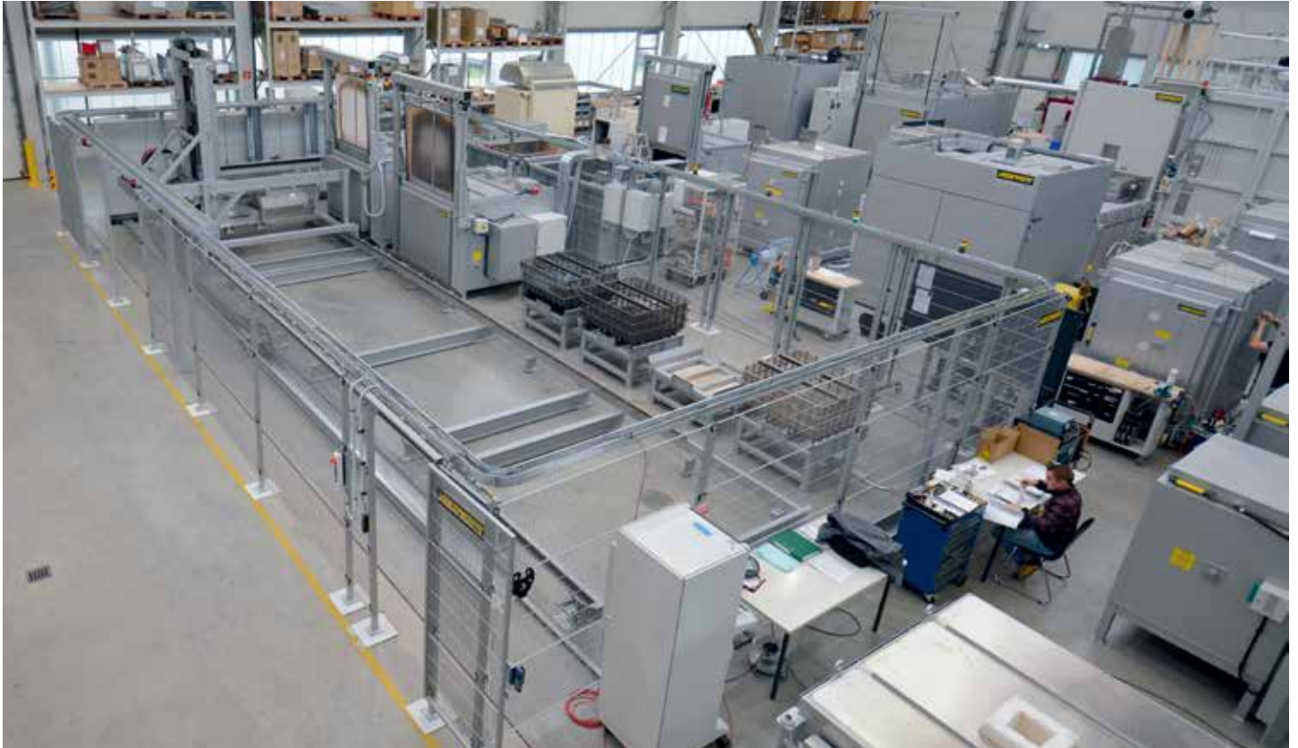
Fully automated tempering plant with two chamber furnaces, quench bath, conveyor system, and parking spots for four charge baskets
