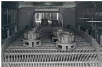
Mesh belt drive in a continuous furnace
